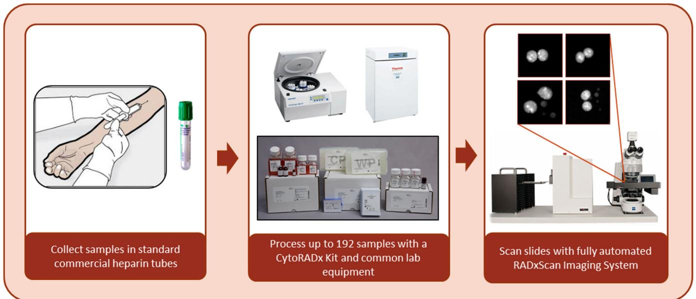
*The CytoRADx™ System combines existing clinical lab equipment with a low-cost assay and the Metafer-based RADxScan automated imaging system to provide high-throughput biodosimetry capability.*
